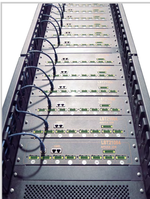
Arbin 96-channel cycler using bipolar circuitry and designed for continuous operation.
