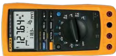
Inadequate meter for calibration
