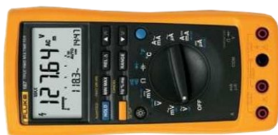
Inadequate meter for calibration
